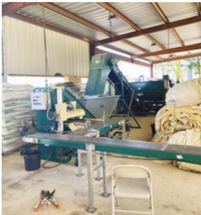
Bracy's Soil Mixture Station amends a composite potting mixture with lime, gypsum, granular micronutrients and a slow-release fertilizer.
